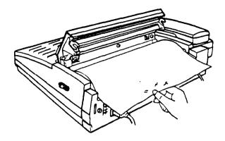
4. Close the cover by pressing down on the center of the cover until it is secure. Tear off the excess paper.
